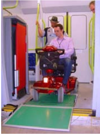
Figure 14 : Mobility scooter trialling wheelchair ramp options on the wooden mock-up
