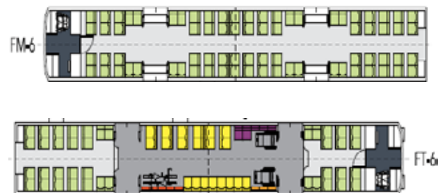
Figure 8 : Finalising the interior layout of motor and trailer cars
