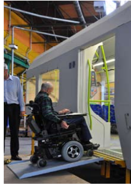
Figure 15 : Smaller powered wheelchair on the timber mock-up
