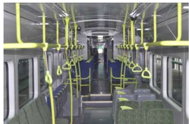
Figure 9 : Unit 1 showing step between low and high floor areas on the trailer car
