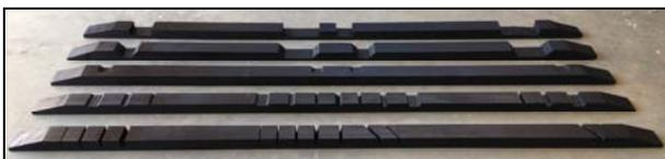
**Figure 12: Wooden carbon strips with simulated defects**
