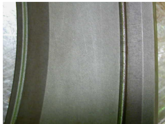
Fig. 6 CTBU class G after 570.000km service backing ring shoulder
