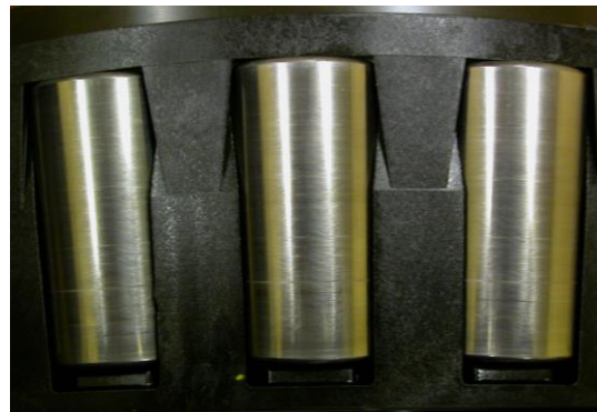
Fig. 8 CTBU class G after 570.000km service bearing cone rollers
