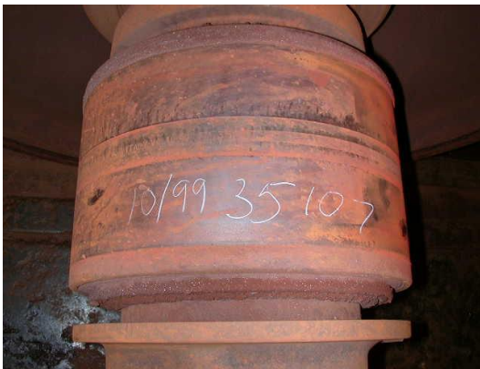
Fig. 5 CTBU class G after 570.000km service before dismantling
