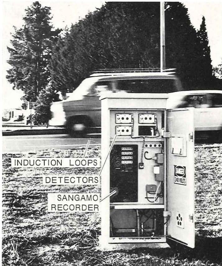
Plate 3—Typical rural counter installation.
