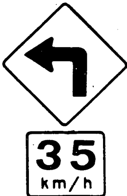
Figure 3 Curve advisory speed sign supplementing curve warning sign (introduced SAA 1975)
